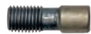
Invisiware® Stud - 3, 11 Non-tensioning inside-the-post-mounted fitting for level or pitched runs swaged on to cable to be used with Invisiware® receiver
