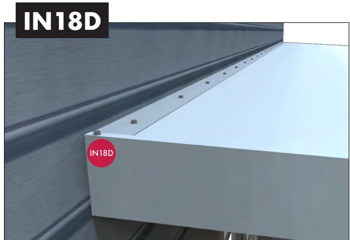
IN18D. Secure side fascia at hanger using 1 ea. Hex Tek #10 x 5/8" fastener: (Part No.: FZ 10X.625 HEXTEK)
