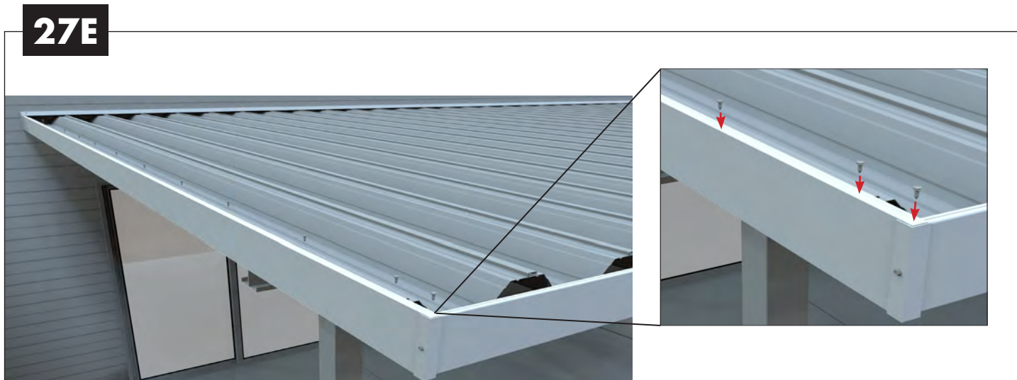
27E. Using Hex Tek #10 x 5/8" fastener (Part No.: FZ 10X.625 HEXTEK) fasten side fascia to the length of the panel every 12-16".
