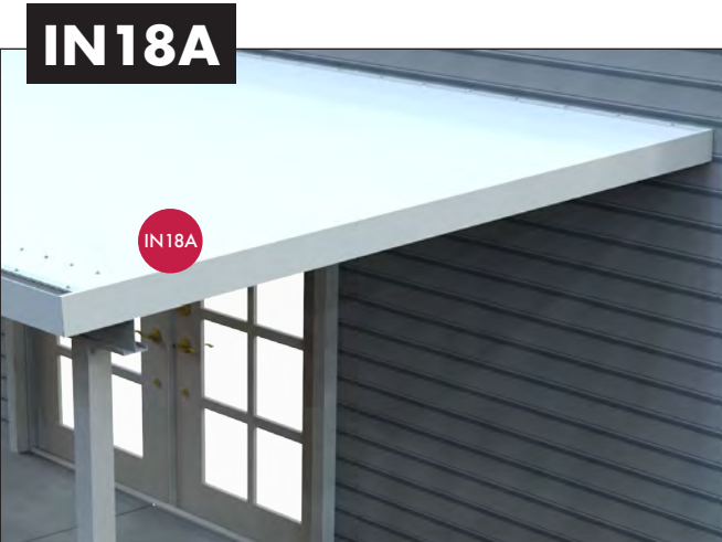
IN18A. Hang the side fascia on top of panel. Ensure top and bottom of side fascia are flush with OU SIDE edge of gutter
