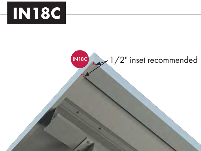
IN18C. Secure side fascia to underside of gutter using 2 ea. Hex Tek #10 x 5/8" fastener: (Part No.: FZ 10X.625 HEXTEK)
