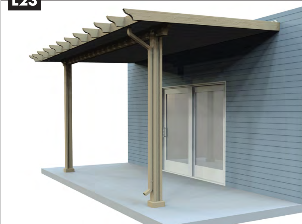
L23. Finished patio cover with lattice wrap.
