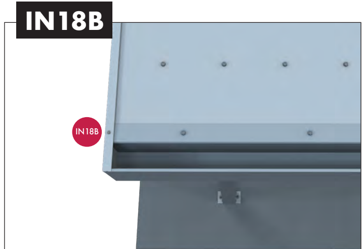
IN18B. Secure side fascia to top flange of the gutter using 1 ea. Hex Tek #10 x 5/8" fastener: (Part No.: FZ 10X.625 HEXTEK)
