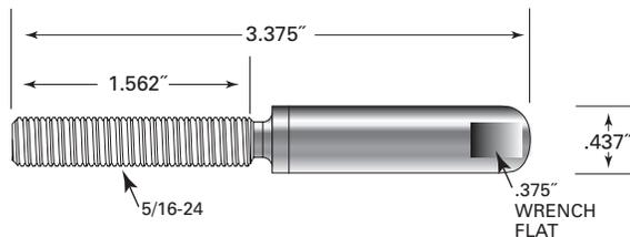
Push-Lock™ swageless studs are made of type 316 stainless steel with the exception of internal components that are made of other types of stainless steel.
