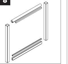
**Measuring and installing picket** or glass/perf vinyl – cut the top rail vinyl for the glass/picket 3" shorter than the top rail – cut the bottom rail vinyl to the length of the bottom rail. Install top and bottom vinyl inside top and bottom rail.
