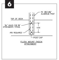
**Fascia mount/flush** – Measure and cut each post to desired length. Insert (2 ea) PIF into the bottom of each post. Cover the bottom of each post with a post cap and using (1 ea)  $\frac{3}{4}$ " painted screw to secure post cap in place. Anchor each post using (2 ea)  $\frac{3}{8}$ " x 7" minimum lag bolts with cap washer and button cap.
