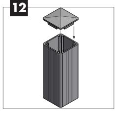
**Install post cap**- Insert post cap into post – secure with one (1 ea) <sup>3</sup>/<sub>4</sub>" painted screw at the top of the post into the tab of the post cap or use silicone sealant.
