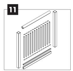
**Installing pickets** – Slide one end of the picket into the bottom rail and swing the other end into the top channel. Push the picket flush and snap on a spacer on each side of the picket. It is necessary to install the last three (3 ea) picket before the spacers. Shift the pickets to allow spacer installation, the last two (2 ea) spacers installed might need to be cut to custom lengths. If necessary, use a rubber mallet to snap spacers into place.
