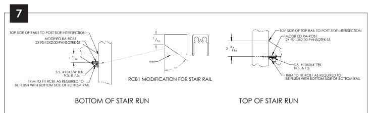
**Rail connecting blocks** – Anchor block into post using #10 x 2" screws (2ea per RCB). Use (1ea) RCB for the top rail and (1ea) for the bottom rail.
