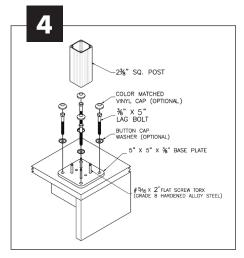
**Surface mount** – Anchor each post using  $(4 \text{ ea}) \frac{3}{8}'' \times 5''$  minimum lag bolts with washers and button caps.
