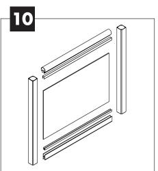
**Installing glass/perf panel** – Wet the top and bottom glass vinyl. Center the glass in the opening betweeen the two posts. Insert the glass into the top vinyl by pushing upwards. Move the **bottom** of the glass **over the bottom rail** and lower into the bottom vinyl.
