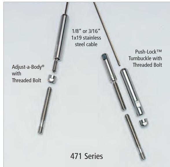
1. Install the tensioning end first with the Adjust-A-Body with Threaded Bolt Tensioner (A-JTB6) by threading the short end of the bolt into the pre-tapped hole in your end post using a 1/4" open-end wrench.
