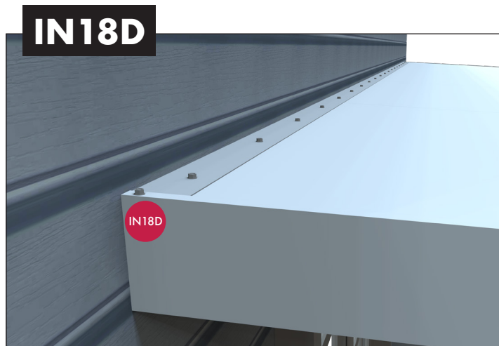
IN18D. Secure side fascia at hanger using 1 ea. Hex Tek #10 x 5/8" fastener: (Part No.: FZ 10X.625 HEXTEK)
